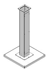
**APPLICATIONS** - Designed for floor mounting of consolets and push button enclosures.
